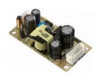
3.3V/1.5A 1.6A 2.0A or 5V/0.5A 1.0A or 6V/1.0A or 12V/0.5A or 15V/0.4A or 24V/0.2A
