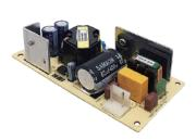
12V/3.8A or 15V/3.0A or 19V/2.4A or 24V/1.9A or 35V/1.3A or 48V/0.93A
